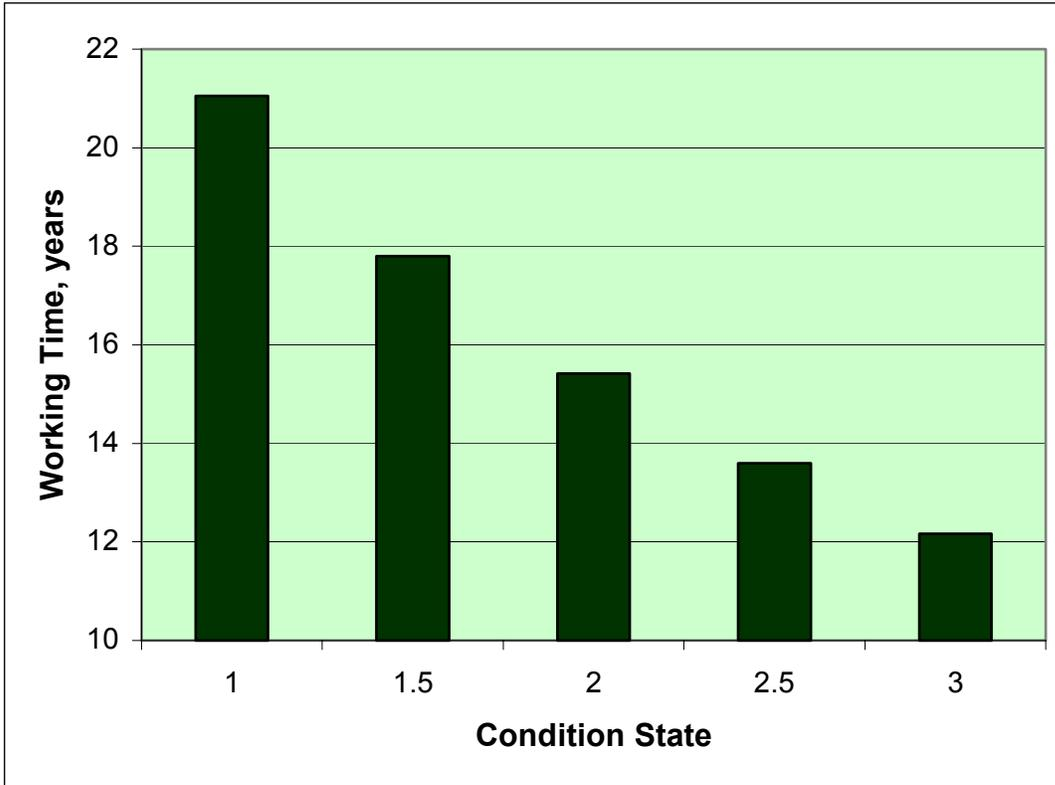
**FIGURE 5 SSE working time in different condition states (an example is SSE #1020 “Reinforced Concrete”)**
